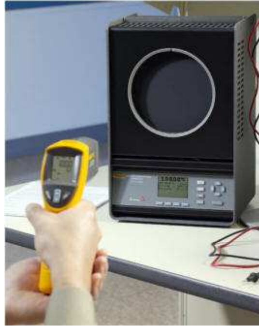
Figure 3. A flat-plate calibrator being viewed by an infrared thermometer. Photo courtesy of Fluke Corporation, Hart Scientific Division, reproduced with permission.
