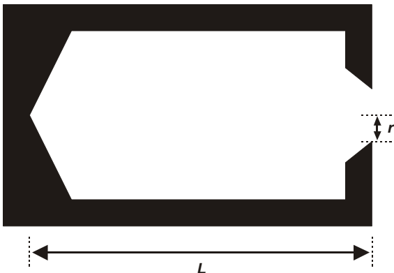
Figure 2. A blackbody cavity of length L and aperture radius r , whose walls have an emissivity \varepsilon_s . The effective emissivity of the cavity is given by equation (10). In use, the cavity is heated uniformly in a furnace or dry-block calibrator.
